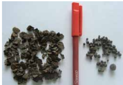
Fig 11: The scale (left) and droplet (right) slags of Nundu ST1.
